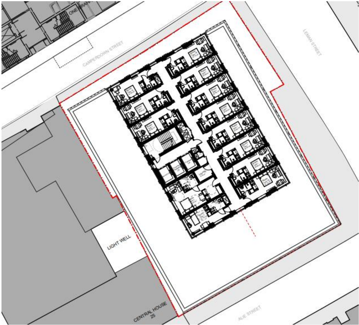
Proposed – Typical hotel floor plan (6-9 th floor)
